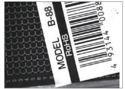
Automatically choosing the most appropriate filter to prevent halation and generating images most appropriate for inspections
